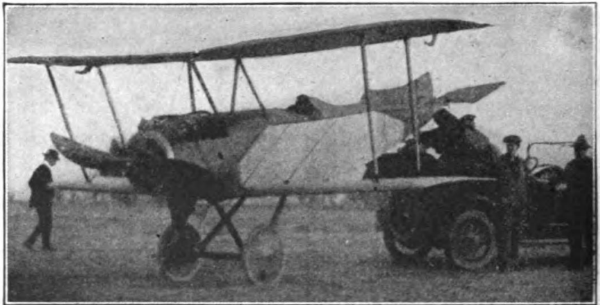
Fig. 1. Curtiss "Baby". Biplane Speed Scout. Equipped with 100 Horsepower Water Cooled Motor.
