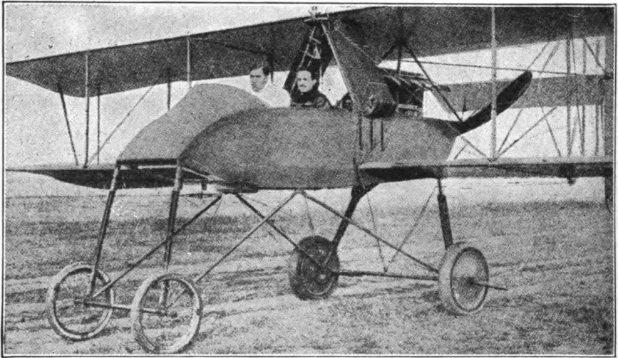
Fig. 6-A. Farman Type Pusher Biplane.... Note the Propeller At the Rear of Body, and the Position of the Pilot and Passenger.
