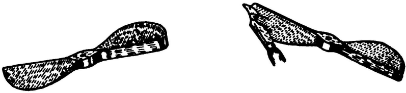
FIG. 41. One blade hollowed. Hollowing the second blade.
